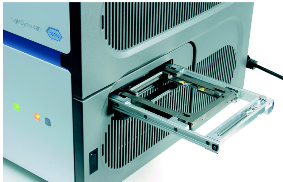
Figure 11: View of an ejected multiwell plate loader
