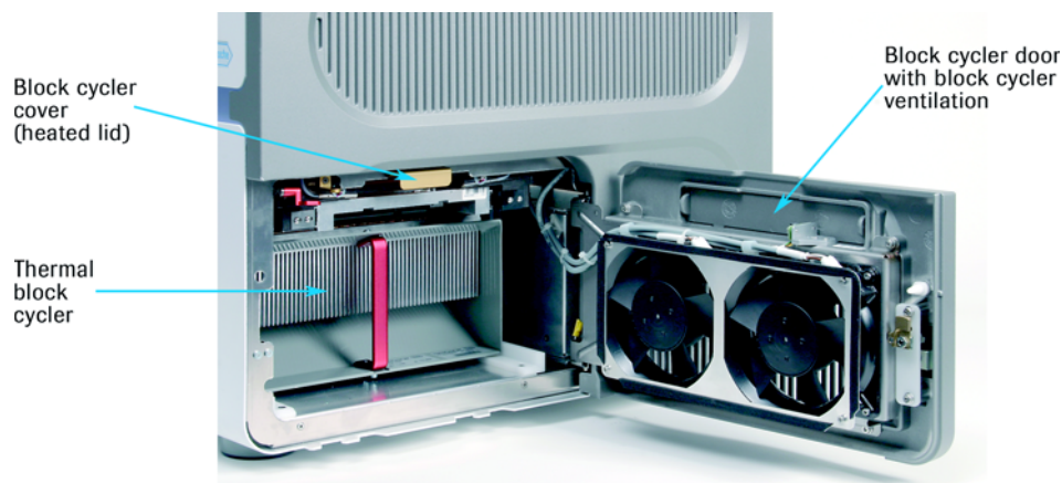
Figure 12: Block cycler door opened allowing a view of the inserted thermal block cycler and block cycler cover
