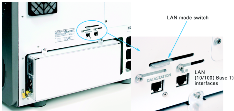
Figure 6: LAN interfaces and LAN mode switch at the rear side of the instrument
