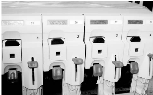
Washblocks disengaged with cartridge levers down
