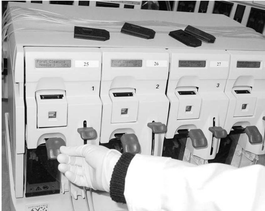
Figure 4.1.5 Remove probe array cartridges and pull up on the cartridge lever to engage the washblock and begin the protocol.
